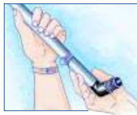
Assembling Poly Pipe: 1. Place clamp over pipe, then insert barb fitting.
