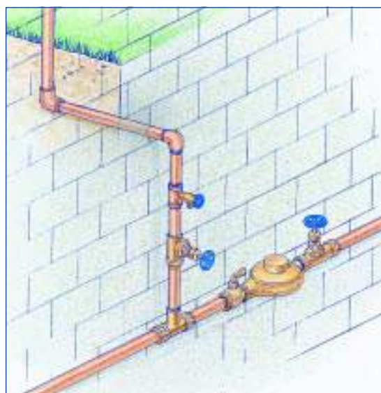
P.O.C. Freezing Climate: If the P.O.C. is in the basement, install a boiler drain immediately after the gate valve to drain the system before the first big freeze.
