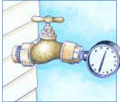
To check water pressure, attach a pressure gauge to the outside faucet nearest the water meter. A pressure gauge can be obtained from your local Hunter dealer.
