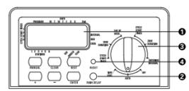
FIGURE 1: Location of Controls on the Timer
