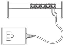
FIGURE 16: Connecting Transformer
